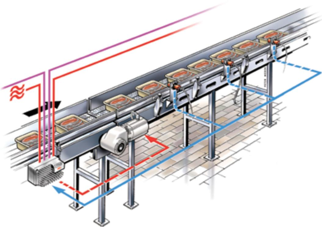
This latest generation VLT® Decentral Drive FCD 302 has been designed with simplicity and robustness in mind and offers significant advantages for multi-motor installations by mounting the drives close to the motors.
